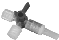
CX-096 Four position valve with two female luer ports (A) and one male luer lock (B)
